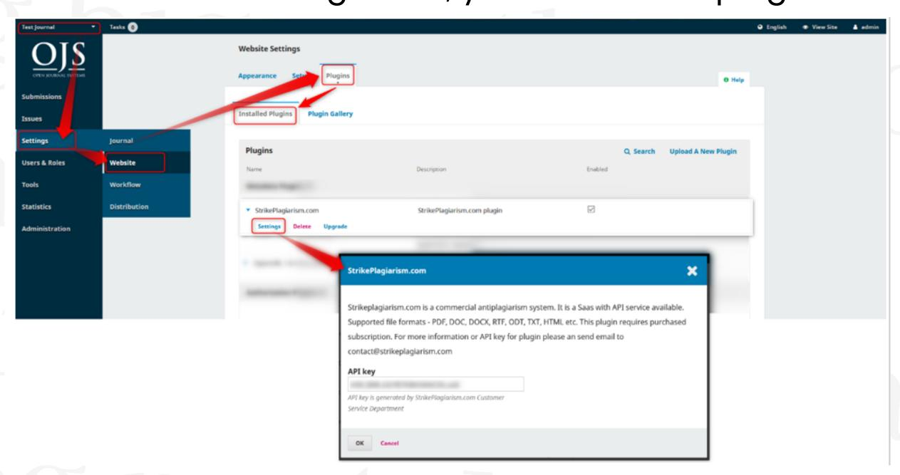
The API key (required for operation of the plug-in), which was sent to you by us should be entered in the plugin settings. After completing above mentioned steps the plugin will be correctly configured, and users will be able to send documents from OJS to anti-plagiarism analysis.
